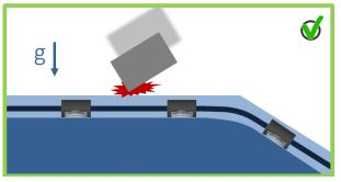
In general, it is recommended to embed the cables in the surrounding construction. For example, the protruding material protects the cable from collisions with other components, e.g. during assembly or maintenance work as well as against falling parts. Especially when routed over edges, the cable otherwise represents an exposed weak point. In addition to sufficient rounding of the edge, attention should also be paid to a suitable cable fastening.
