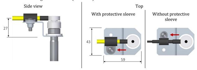
For PB16: Bracket set for signal cable LC16 (04.10016)
