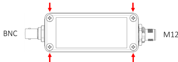
Figure 2: Fastening screws on the cover
